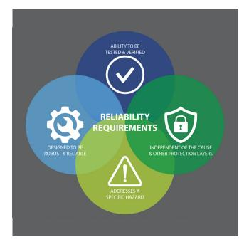
In a manufacturing facility, protections are implemented to prevent or minimize hazards identified in a risk assessment. A protection in a basic process control system (BPCS) that meets the following core requirements is considered an Independent Protective Layer (IPL):
